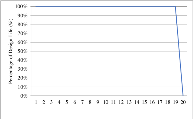
Images 1 Graph of Declining Design Life in Normal Conditions Based on Bina Marga (1987)
