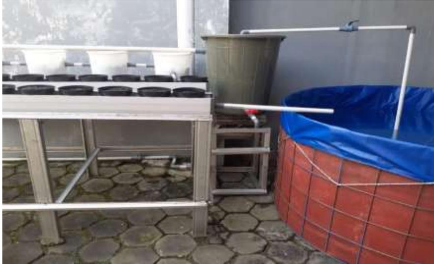
**Gambar 4. Unit kolam Bioflok-Aquaponik**
