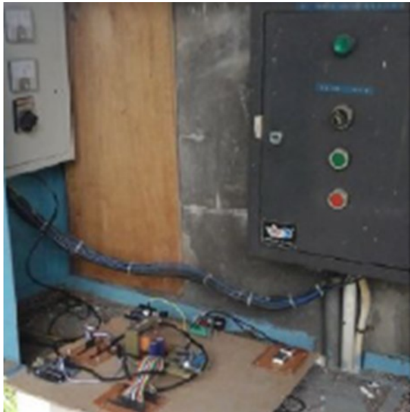
Fig. 12. The circuit controller with microcontroller arduino uno.
